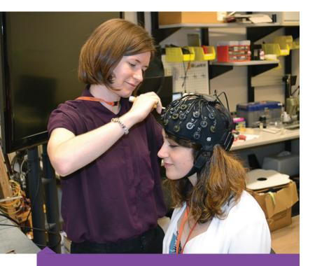
Kaela Shea, EIT (left), a PhD candidate who conducts research at PRISM lab at Holland Bloorview Kids Rehabilitation Hospital, sets up a functional near-infrared spectroscopy system for a feasibility test of data collection with summer intern Laura Wheeler.
