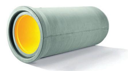
PERFECT PIPE, a concrete pipe product manufactured with a high density polyethylene (HDPE) liner and thermoplastic internal connectors with dual elastomeric rubber gaskets for the ultimate in joint integrity and durability. It's the future of waste water systems and it's only available in Canada through Con Cast Pipe. Contact us to learn more or for a plant tour to view the production of the PERFECT Pipe.
