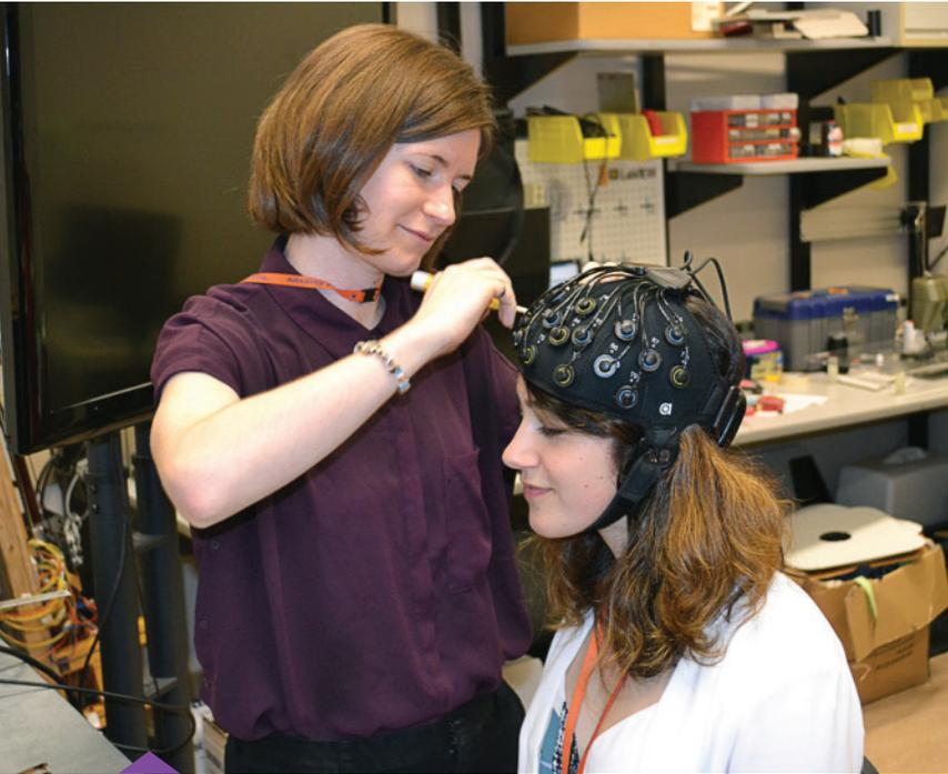
Kaela Shea, EIT (left), a PhD candidate who conducts research at PRISM lab at Holland Bloorview Kids Rehabilitation Hospital, sets up a functional near-infrared spectroscopy system for a feasibility test of data collection with summer intern Laura Wheeler.
