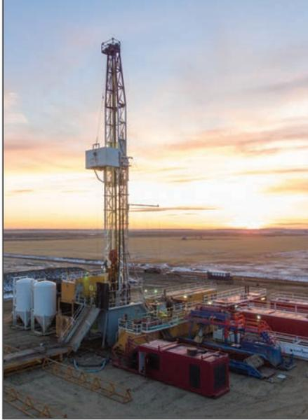
DEEP has five drilling projects located in southern Saskatchewan, including this drill, located outside of Torquay, which has reached a depth of over 3500 metres to source geothermal energy from a heated aquifer.
