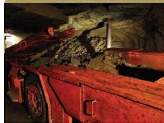
Cut and fill stoping is an underground mining method in which the ore body is retrieved in horizontal slices starting at the bottom and working upwards towards the surface. Ramps are
