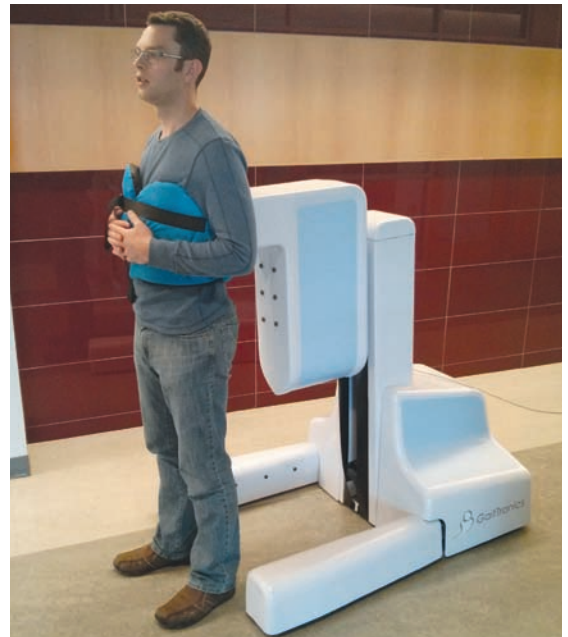
Richard Beranek, CEO of GaitTronics, demonstrates GaitEnable, a robotic device that helps patients walk unassisted following surgery or during physiotherapy.
