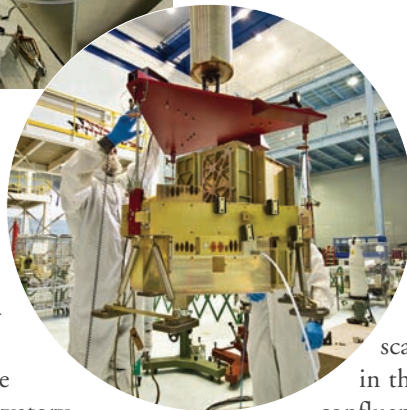
The FGS/NIRISS, the Canadian component of the James Webb Space Telescope, is getting a lift in the giant clean room at NASA Goddard Space Flight Center. In this photo, the FGS/NIRISS was being lifted for placement on a master tool for key measurements prior to installation onto its flight structure later. Photo: NASA Goddard/Chris Gunn
