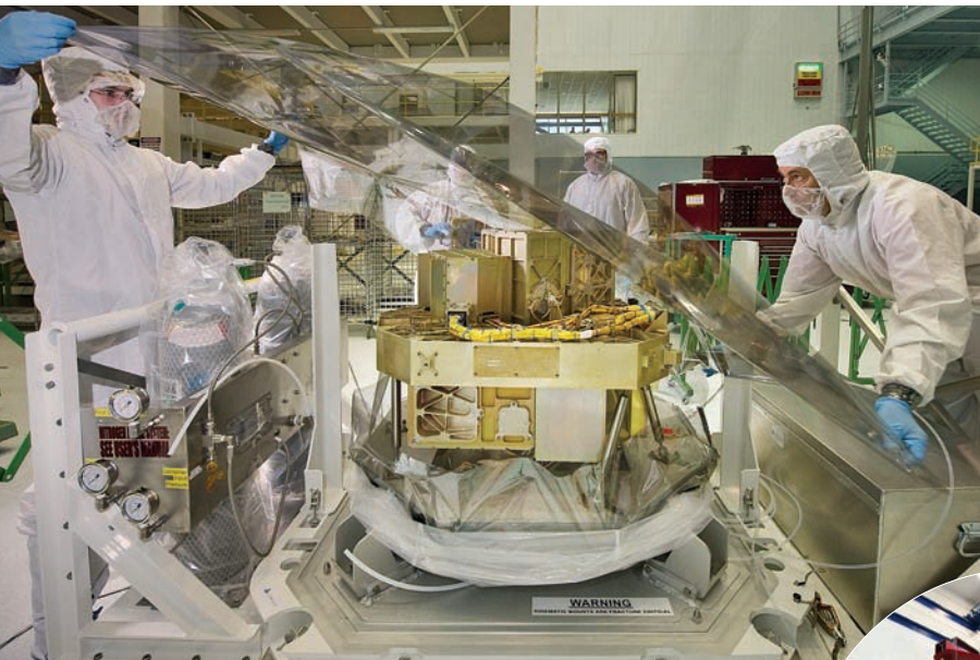
After performing an initial post-shipping inspection of the James Webb Space Telescope's FGS/NIRISS in a clean room at NASA's Goddard Space Flight Center, engineers from COM DEV and NASA place a protective drape over the instrument until work resumes the next day. Photo: NASA Goddard/Chris Gunn
