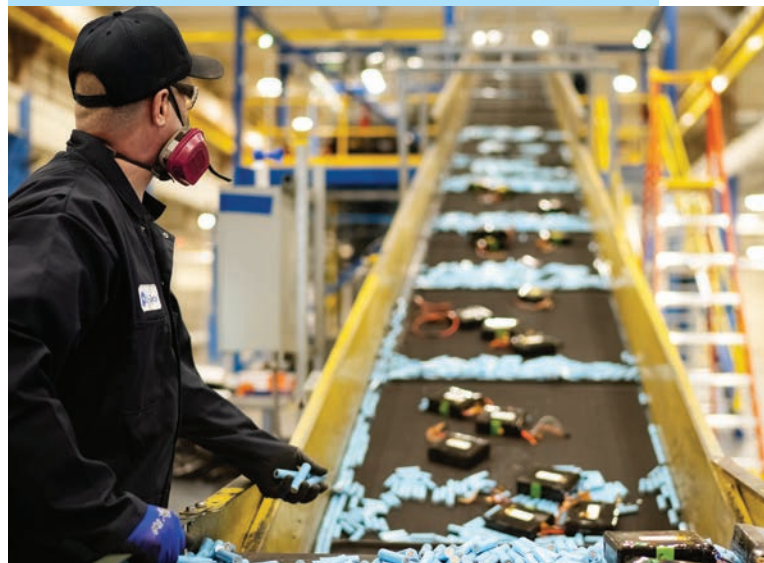
A Li-Cycle employee manages lithium-ion batteries on a conveyor belt at the company’s Rochester, NY, spoke. Photo: Li-Cycle
