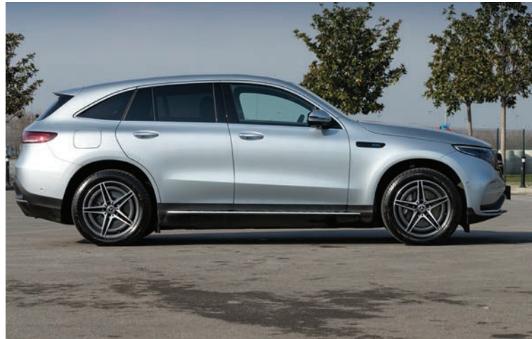
The Mercedes Benz EQC is a fully electric vehicle powered by a lithium-ion battery weighing 650 kilograms when introduced in 2018.
