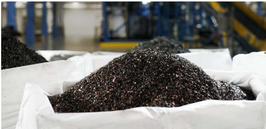
An image of black mass, containing nickel, cobalt and lithium in its pure form. Unlike earlier processes, Li-Cycle is able to retrieve them without using any thermal or treatment processes.
