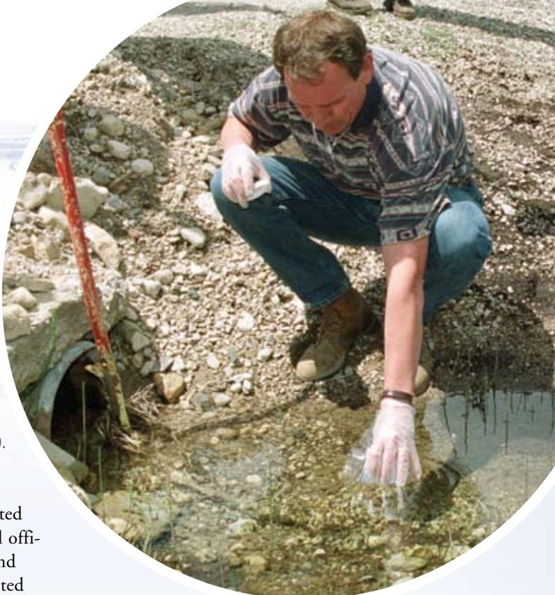
Greg Powers, a regional groundwater officer, Ontario environment ministry, draws a sample of groundwater from a culvert next to one of the wells feeding the Walkerton water distribution system. The Ontario environment ministry implemented compulsory water testing and has drawn up new standards for measuring contaminants and disinfection levels as part of its multi-level response to the Walkerton disaster of May 2000.
