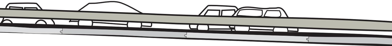
glass are placed within the steel frame and the entire structure is infused with thermosetting resin, creating a monolithic structure. Together, such a combination of materials reduces dead loads (bridge weight) by approximately 20 to 30 per cent.
