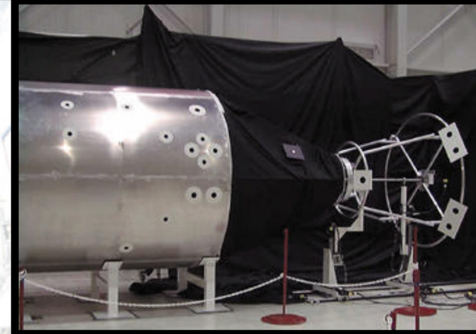
**Getting ready for space flight:** One of several half-scale models of International Space Station payloads used to verify space operations at Neptec's Vision Systems Certification Lab. Mounted on platforms, the models stimulate the movement of payloads in space, making preflight testing as realistic as possible.
