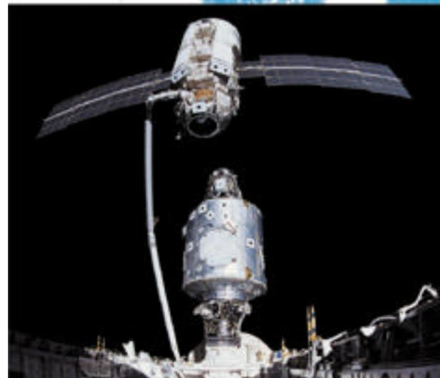
Neptec's space vision system was used during mating of the Russian Zarya module (top payload) and the American Unity module (bottom payload). Zarya will provide propulsion control, power and fuel storage throughout the early stages of assembly, while Unity will serve as a juncture point for six critical station components, including the U.S. Laboratory and U.S. Habitation Module.
