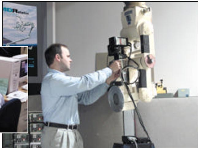
**In the space lab: Ross Gillett mounts the 3-D imaging camera, part of a robotic system prototype for missions in space.**
