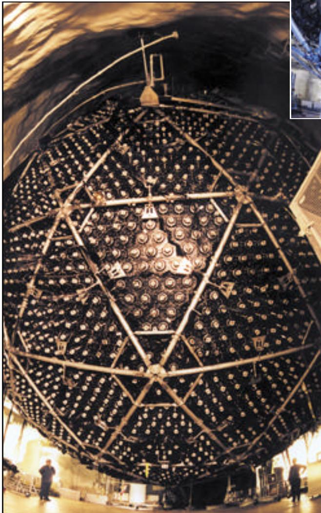
**A window on the cosmos:** The Sudbury Neutrino Observatory's support structure holds hundreds of photomultiplier tubes that detect faint flashes of light as neutrinos collide in heavy water.
