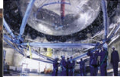
**Inside the SNO cavity:** 2 km beneath the Earth's surface, the acrylic vessel holds heavy water to detect mystery neutrinos.
