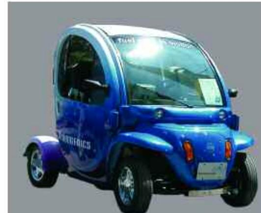
Powered by a hydrogen fuel cell, the Hydrogenics GEM car is a small, neighbourhood electric vehicle. The GEM car can reach speeds of 25 km/h and is environmentally friendly, since water is the only emission.
