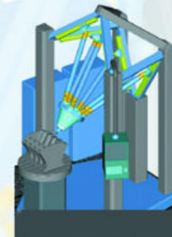
The TIARA hexapod is a high-speed, high-performance machine tool currently under development at the Intelligent Machines and Manufacturing Research Centre in Hamilton.
