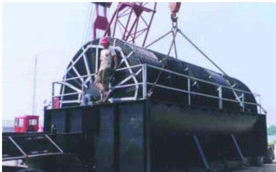
No contamination: A Rotating Biological Contactor built by CMS Group Inc. can help protect the water table.
