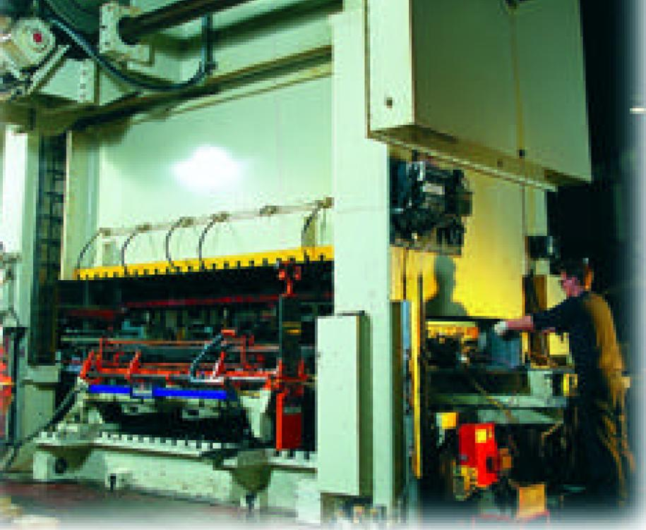
◀ A plant worker at Triton Manufacturing in Mississauga uses a transfer press to stamp out auto parts. Triton is currently in the process of obtaining ISO 14001 certification.
