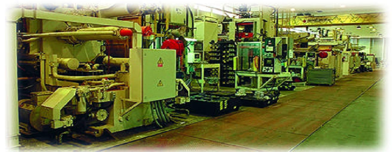
▲ High pressure die casting machines produce magnesium parts at Meridian Technologies Inc.'s Strathroy, Ontario, division.
