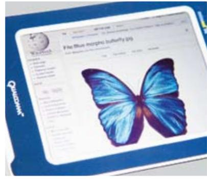
Qualcomm's new mirasol technology is the first full-colour, video-capable display on a prototype e-book reader (right). Built on the concept of the iridescence of a butterfly's wing (left), the technology reflects light rather than transmitting it the way LCD screens do.
