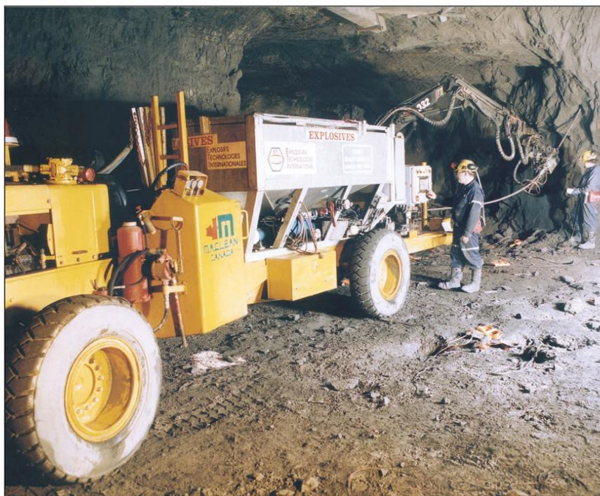
Workers at Brunswick Mining and Smelting manually load explosives into production holes, using a Maclean emulsion loader. Maclean and several partners are working on a project to automate this dangerous process.
