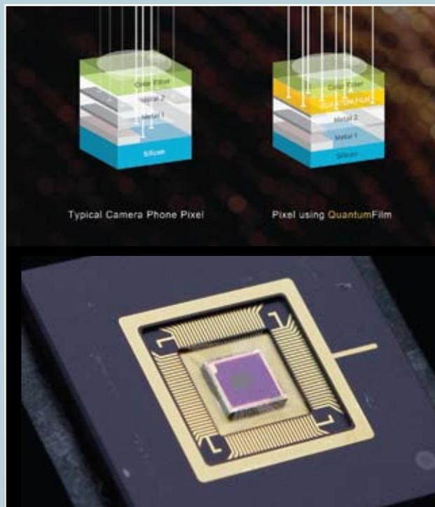
This graphic prepared by InVisage Technology shows the enhanced light capturing ability of QuantumFilm compared to traditional silicon-only digital imaging systems. The world’s first image sensor using quantum dots will bring high-quality images to cellphones.
