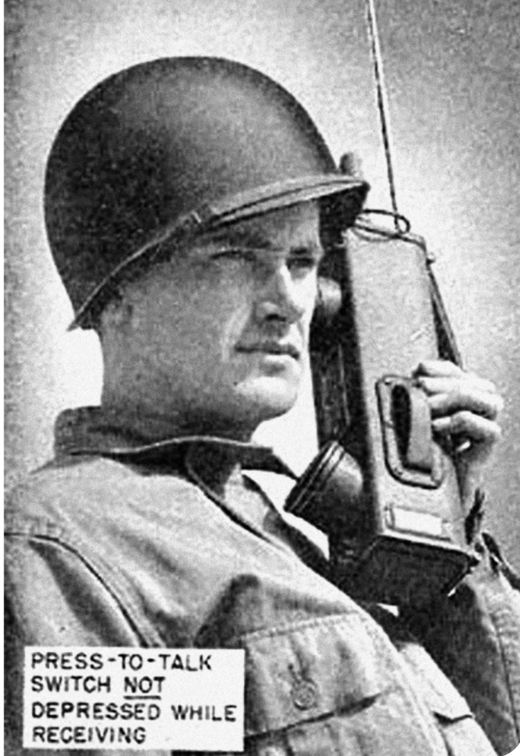
A SCR-536 US military "handie talkie," the first hand-held walkie talkie, which was developed three years after Hings'
