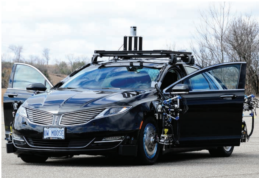
The Autonomoose is a Lincoln MKZ hybrid sedan that has been modified with artificial intelligence to become a self-driving car.
